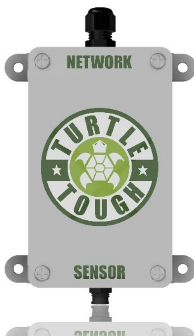
Figure 3-1 — The Integration Module (TT-ISO-DSS-DC). Orderable in two enclosures: TT-ISO-DSS-DC-IP67 (IP67, cable glands, panel-mount female sensor connector) and TT-ISO-DSS-DC-DIN (DIN-rail, IP44, sensor input loom). Both are blind (no local display), accept 9–36 V DC input and output isolated MODBUS RTU.
