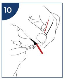
Cut the capillary tube on an angle
