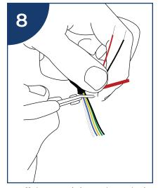
Cut off the remaining coloured wires
