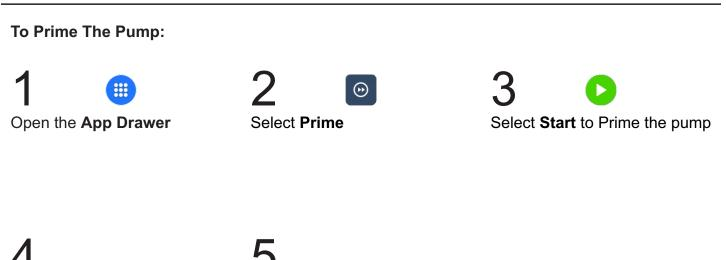
Pump will run at 100% motor speed for sixty seconds
