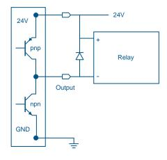
Fig. 5: Connecting Output Q1 to Relay
