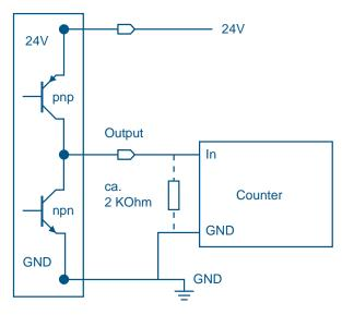
Fig. 6: Connecting Output Q2 to counter
