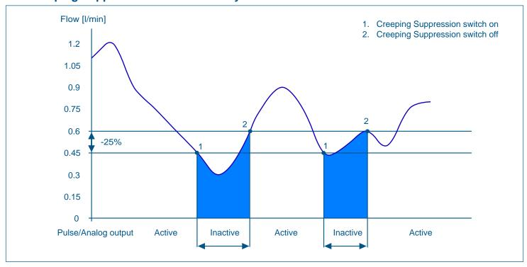
Fig. 7: Function of the creeping suppression illustrated with 0.6 l/min
