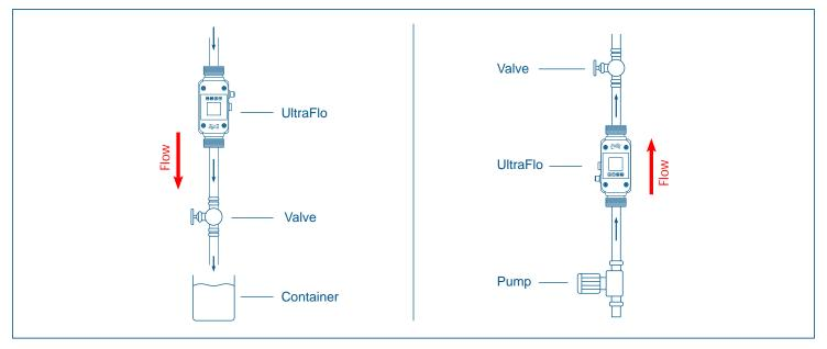
Fig. 3: Mounting examples for UltraFlo
